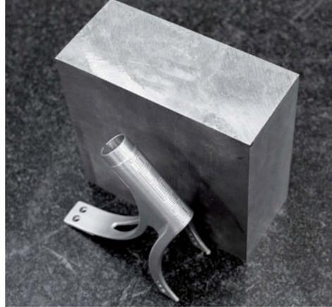
Seat Post Alongside Billet to Demonstrate Rough Machining
