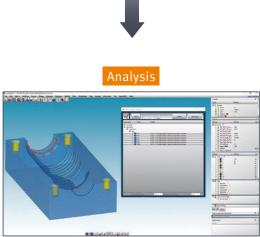
■ Check the quality of faces/solids ■ Find double entities ■ Range of analysis functions: Draft angle, undercuts, radii, spherical face analysis, and so on
