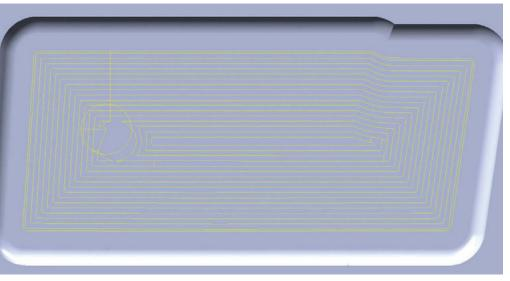
hyperMILL® MAXX Machining roughing module Tool Path on Pocket
